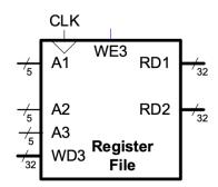
You may assume that this register file is implemented using **positive edge-triggered D** flip-flops.
